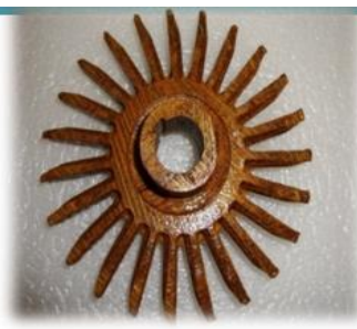
Epoxy coated impeller
